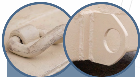
TWO 26,500lb RATED D RINGS AND REAR TOW CONNECTION
